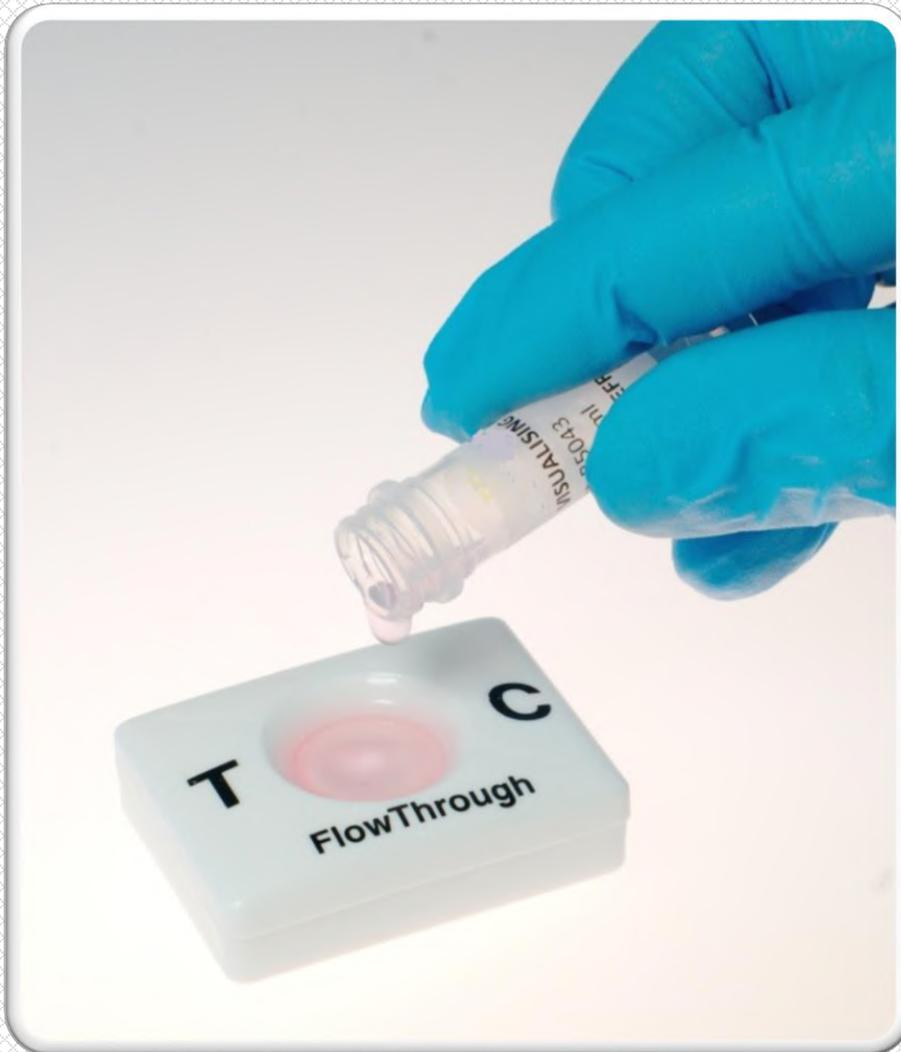
**Qualitative test for on-site detection of gluten
